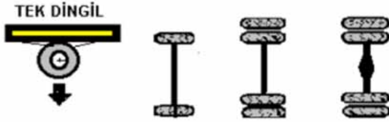
Şekil 4: Dingil 12 ton, Tek tekerlek 6 ton / Figure 4: Axle 12 tons, Single Wheel 6 tons
